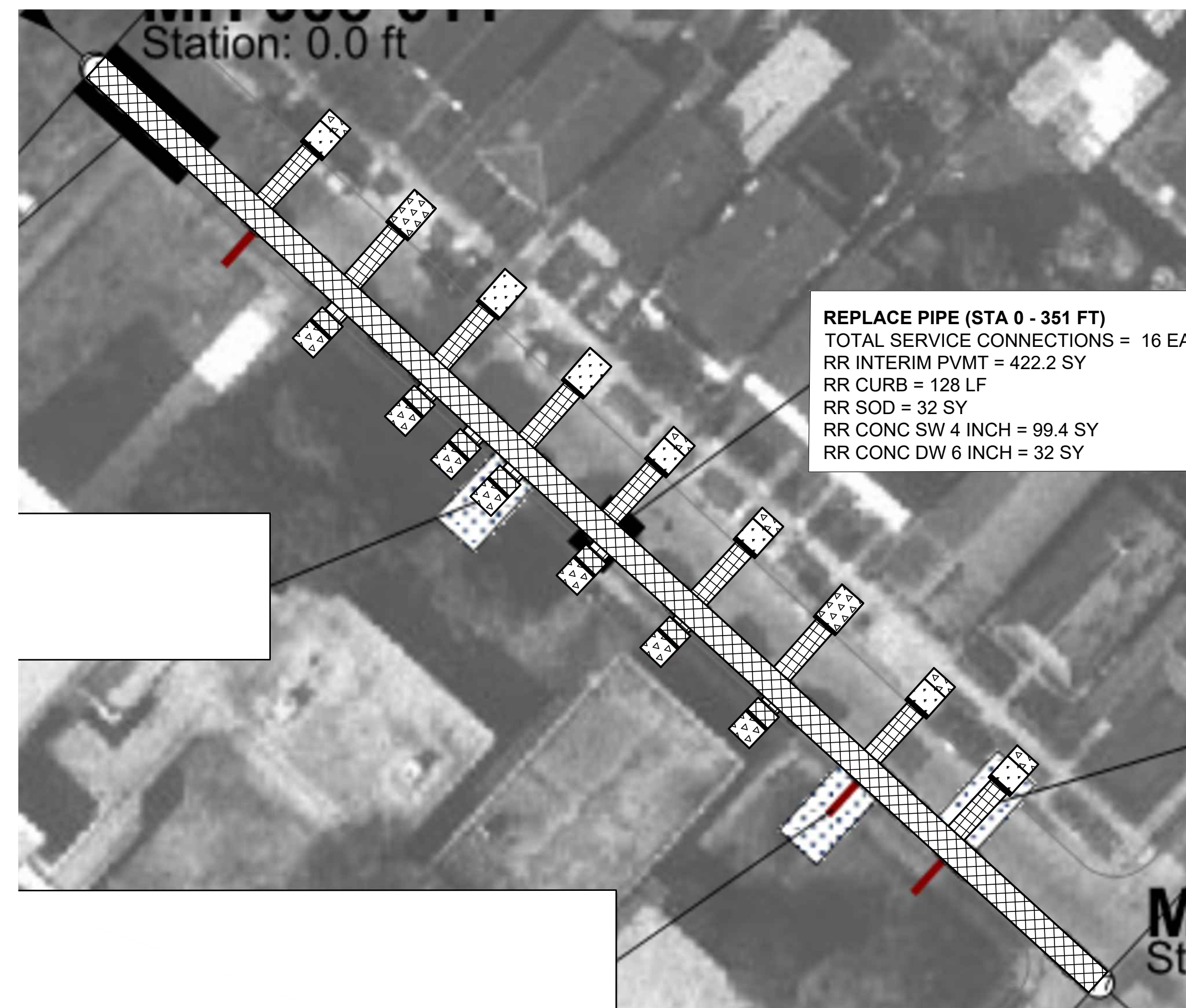
SSERP ROADWAY RESTORATION FORSHEY ST (9300) NTS NOTE: PAVEMENT RESTORATION FOR THIS ROADWAY SHALL BE "INTERIM PAVEMENT" AS SCHEDULED IN THE SPECIFICATIONS. PERMANENT SITE RESTORATION, INCLUDING INTERSECTIONS, TRANSITIONS, AND ADA RAMP, WILL BE PERFORMED UNDER DPW CONTRACT RR218. SIDEWALKS, DRIVEWAYS AND SOD SHALL BE RESTORED IN ACCORDANCE TO DPW STANDARDS. OTHER WORK ON THIS BLOCK MAY BE PERFORMED UNDER DPW RR218. CONTRACTOR SHALL COORDINATE THIS WORK PRIOR TO FINAL PAVEMENT RESTORATION.
